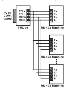
3.TMC-03 Full-duplex communication connect between Interface converter
